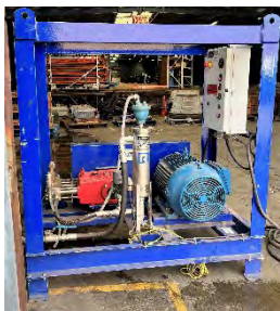
HIGH PRESSURE (12500PSI) WASHER BLASTER
