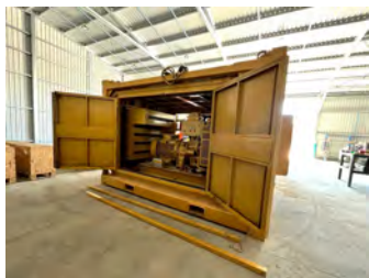
DIESEL GENERATOR 80kVA/50Hz ZONE 2 RATED
