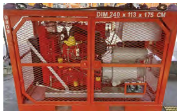
AIR COMPRESSOR 190CFM ZONE 2 RATED
