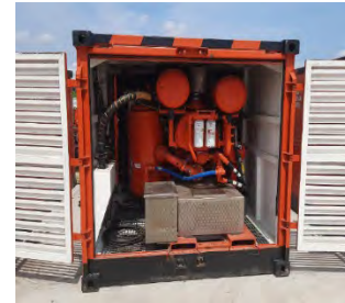
900 CFM RIG SAFE 150PSI AIR COMPRESSOR
