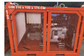
GENERATOR 32KW ATEX ZONE 2 IECex CERTIFIED
