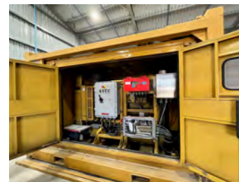
DIESEL GENERATOR 30KVA ZONE 2 RATED
